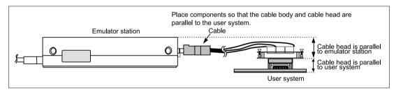
Figure 11 User System Interface Cable Location Example
